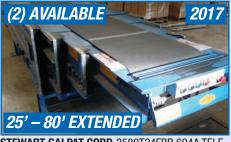
STEWART GALPAT CORP. 2580T24FBR 694A TELE-SCOPING EXTENDABLE TRIPLE BOOM CONVEYOR
